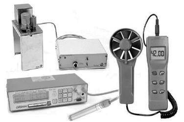
**Fig.1.** Equipment used in the experiment: portable dust monitor (left down); dust generator (left up); portable anemometer (right)
