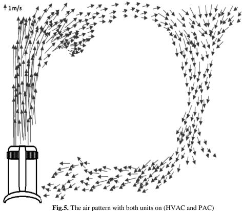
**Fig.s.** The air pattern with both units on (HVAC and PAC) – velocities less than 0.5 m/s were not included
