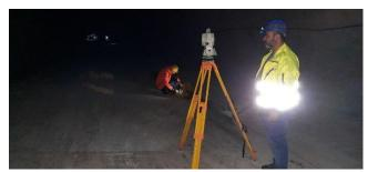
Fig. 3. Positioning geophones
