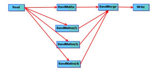
**Fig.2.** Graph Builder -Band Math 1 NDWI (B3-B11)/(B8+B11), Band Maths2 MNDWI (B3-B11)/(B8+B11), Band Maths3 MNDWI5 (B8-B4)/(B8+B4), BandMaths4 AWEI B2 + 2.5 \* B3 - 1.5 \*(B8-B11) - 0.25 \* B12
