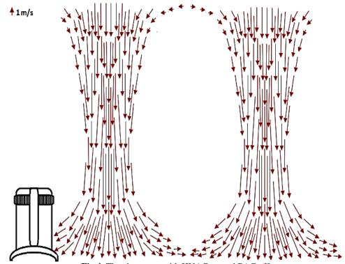
**Fig.4.** The air pattern with HVAC on and PAC off (velocities less than 0.5 m/s being were not included)
